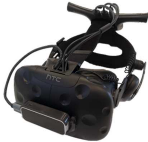
Figure 1. HTC VIVE glasses with Leap Motion.
