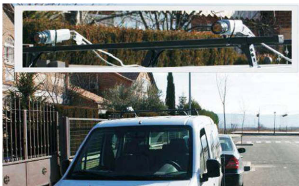
Fig. 2. Acquisition subsystem: two cameras on the top of the van.
