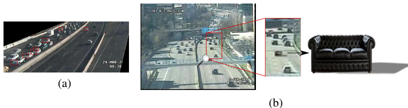
Fig. 2. (a) Results of the HOG detector [6] in a traffic congestion image. (b) In these images the vehicles typically occupy a few pixels, and it becomes difficult to identify the typical cues that we use for finding cars (e.g. wheels, license plates). Instead, note that the context results fundamental to determine whether a blob represents a car or a black couch, for example.
