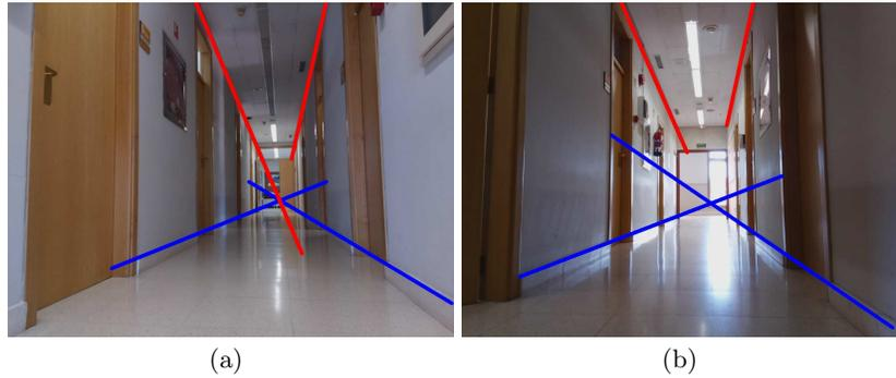
Fig. 5. Examples of detection of wall-floor and wall-ceiling boundaries.
