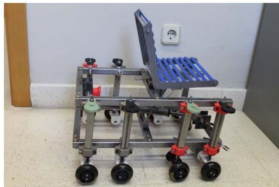
Figure 17: First built prototype (1:2 scale). Main structure. All components, except the electrical motor and the pulley belt transmission system, have been designed, developed and built in our laboratory.
